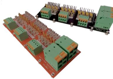
The RapidFuse Board is built from extremely high quality PCBs, heavy copper pours (to minimize voltage drop, heat, and resistance), and the best Phoenix connectors available for the application. These boards are not designed to be cheaper than an AGC fuse row, these are designed to be better and much faster to install.
